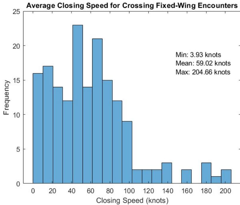
Figure 57. Average Closing Speed for Crossing Fixed-Wing Encounters.
