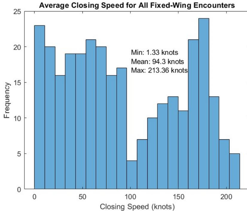
Figure 55. Average Closing Speed for Fixed-Wing Encounters.
