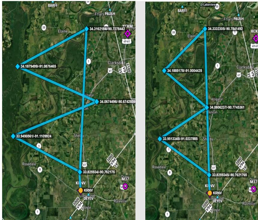
Figure 24. Butterfly wing flight paths used for overtakes.
