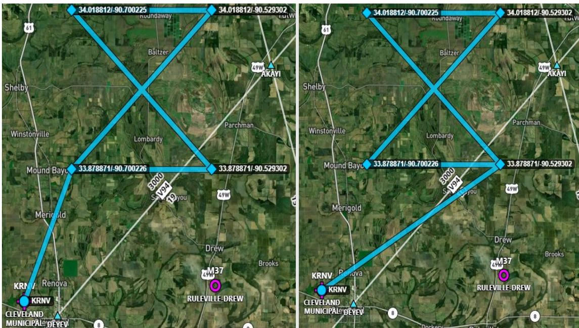
Figure 20. Hourglass flight path with near 90-degree variation.
