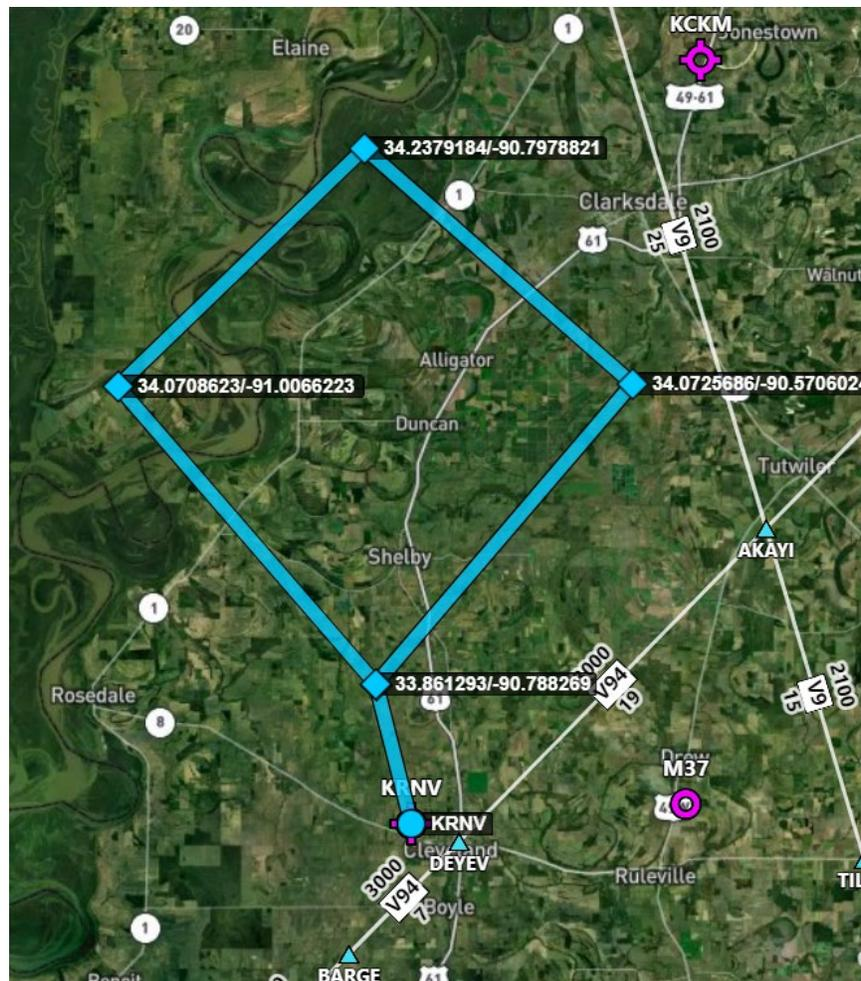
Figure 25. Intruder diamond flight path for overtaking encounters.
