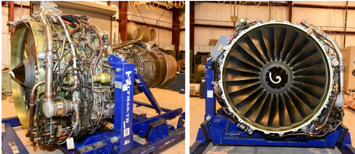
Figure 23. CFM56-7B engine used for ingestion test.
