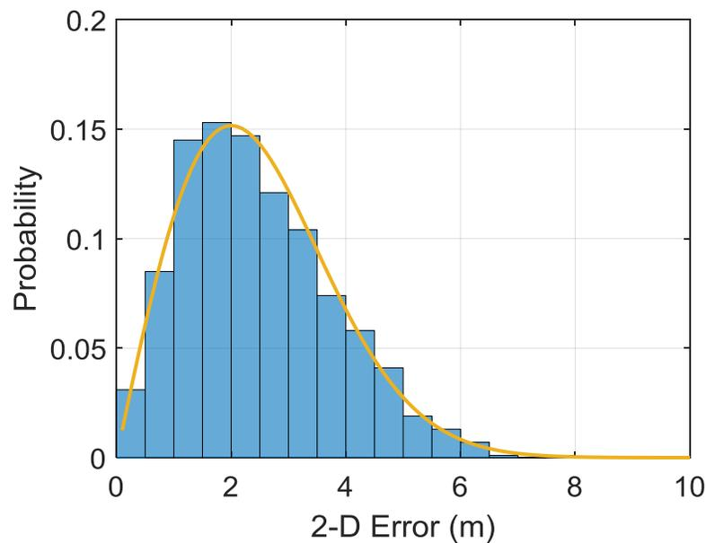
**Figure 5.1. 2D GPS error distribution**
