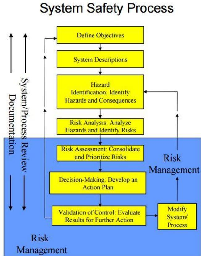
**Figure 5.2. SRM System Safety Process**
