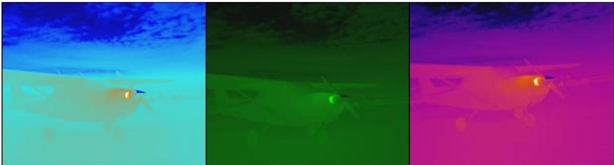
**Figure 6.12. Three different color schemes on the FLIR thermal camera showing the same aircraft pictured in Figure KK. Note the bright area showing the warm engine in the front of the plane. By using false color representations, select characteristics may be highlighted with the thermal imagery.**
