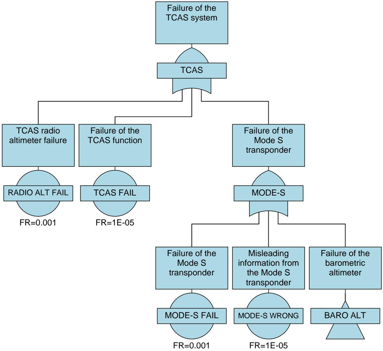
**Figure 5.8. TCAS failure tree**
