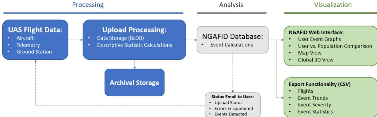
Figure 8. NGAFID Data Flow Diagram.
