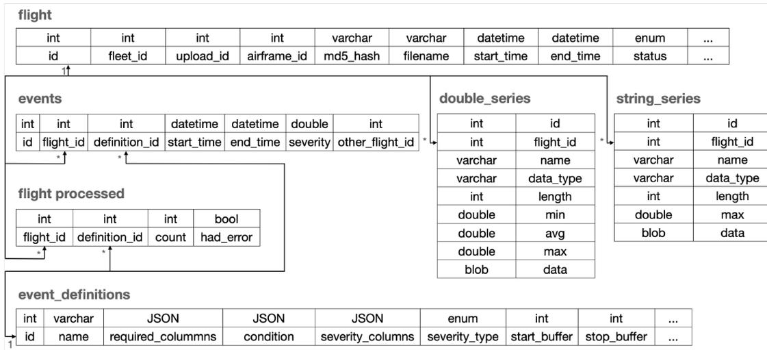
Figure 7. Schema for Data Processing in the NGAFID.
